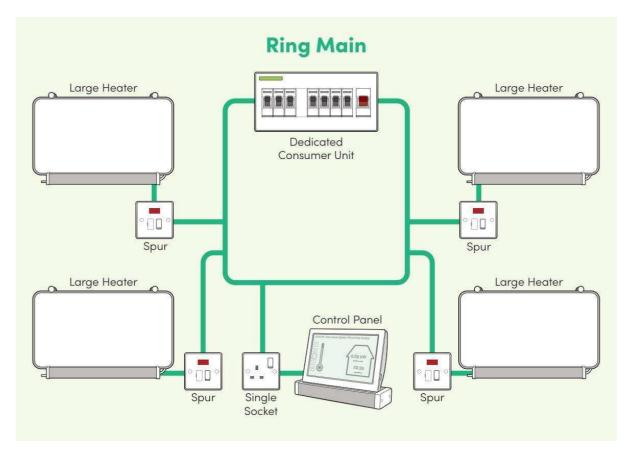
A floorplan will be provided showing the heater locations and the type/size of the heater to be installed. Ensure that the fuse spur will not be sited behind the heater when it is in its installed position. The fuse spur should be positioned to the right of where the heater will be located if possible. Each heater has approx. 1.5m of flex exiting from the lower right side of the base.
