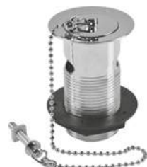
1 1/4" basin waste, slotted, brass bodied, metal plug, brass backnut – chrome-plated C50021
